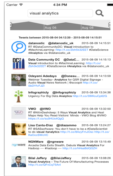
Figure 1: The simple search mode provides a query box and search results list, as well as a timeline visualization.
