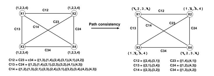
Figure 5: Applying a path consistency algorithm to the 4-queens problem .
