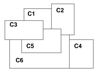
Variables: {Q1,Q2,Q3,Q4} Domain: {1,2,3,4} Constraints: {Qi <> Qj , |Qi-Qj| <> | i - j | } Variables: {C1,C2,C3,C4,C5,C6} Domain: {R,G,B} Constraints: {C1 <> C2, C1 <> C3 ....}
