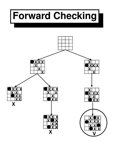
Figure 7: Applying Forward checking to the 4-queens problem
